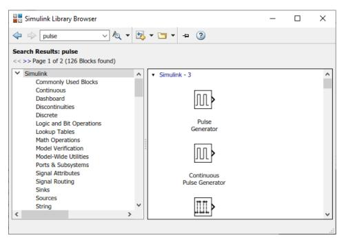
Get detailed information about a block. Right-click the Pulse Generator block, and then select **Help** for the Pulse Generator block. The Help browser opens with the reference page for the block.
