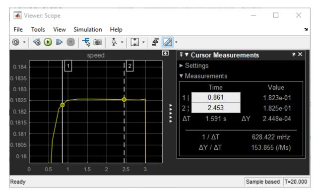
The **Value** column in the **Cursor Measurements** panel indicates that the top speed of the robot is 0.183 m/s. To calculate the time it takes for the robot to travel 0.05 m, divide 0.05 m by 0.183 m/s. You get 0.27 sec.
