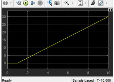
This simulation shows that the angle increases steadily when the wheels are turning with the same speed in opposite directions. You can make some model improvements to make it easier to interpret the angle output, for example:
