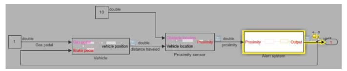
**3** To continue tracing the signal to its source, press the left arrow key.
