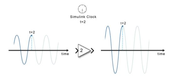
In simulation, time progresses differently from a real clock. Each time step takes as much time as it takes to finish the computations for that time step, whether that time step represents a fraction of a second or a few years.
