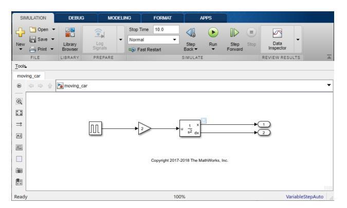
Simulating this model integrates a brief pulse twice to get a ramp. The results display in a Scope window. The input pulse represents a press of the gas pedal -1 when the pedal is pressed and 0 when it is not. The output ramp is the increasing distance from the starting point.
