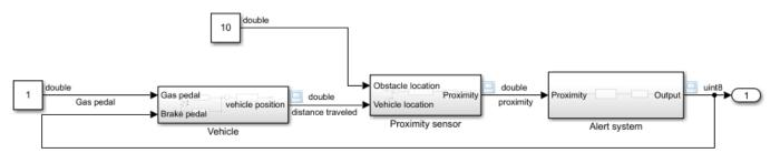
The model displays data types along the signal lines. Most signals are double, except the output of the Alert system. Double-click the subsystem to investigate.
