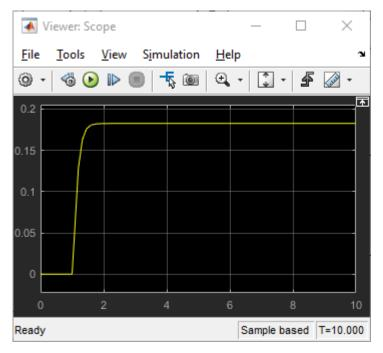
The simulation result exhibits the general expected behavior. There is no motion until force is applied at step time. When force is applied, the speed starts increasing and then settles at a constant when the applied force and the drag force reach an equilibrium. In addition to validation, this simulation also gives information on the maximum speed of the wheel for the given force.
